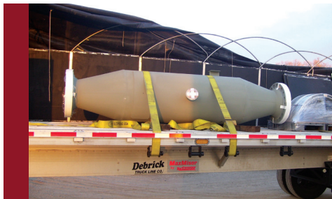
Horizontal Vortex Scrubber
